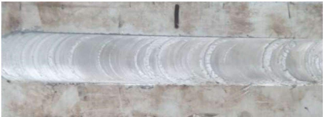
Figure 4 Crown appearance of friction stir processed specimen
